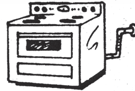
20. gas stove with rigid feed line
